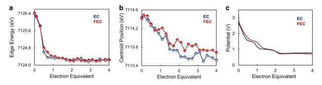
Figure 8: (a) Fe K-edge energy and (b) centroid position of the pre-edge peak as a function of electron equivalents with (c) corresponding electrochemistry of operando Li/Fe<sub>3</sub>O<sub>4</sub> cells with EC (blue) and FEC (red) electrolyte.
