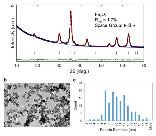
Figure 3: Characterization of Fe<sub>3</sub>O<sub>4</sub> nanopowder. (a) Rietveld refinement of the XRD pattern with reflection lines. Black represents the observed pattern, red is the calculated fit, green is the difference, and blue represents background. (b) TEM image and **c** particle size distribution statistics.
