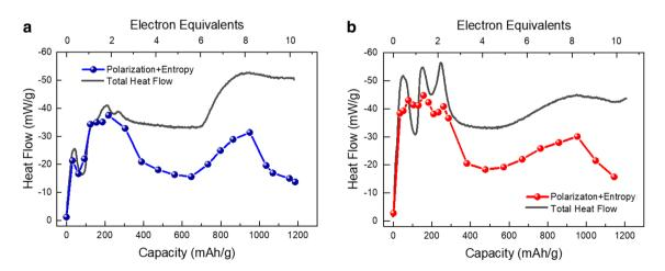
**Figure 6:** Comparison of total heat flow from IMC (gray, solid line) and experimentally determined polarization and entropic heat flow contributions during lithiation in the presence of (a) 1 M LiPF6 EC/DMC (3/7 v/v) (blue, connected-dot line) and (b) 1 M LiPF6 FEC/DMC (3/7 v/v) (red, connected-dot line).
