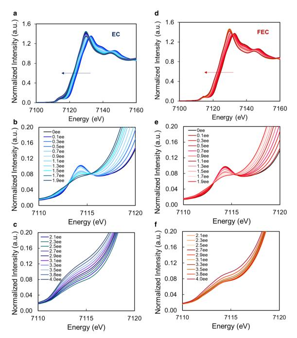
Figure 7: XANES spectra of Li/Fe<sub>3</sub>O<sub>4</sub> operando cell with (a)–(c) EC and (d)–(f) FEC electrolyte with highlighted pre-edge feature from (b), (e) 0 to 1.9 ee and (c), (f) 2.1 to 4.0 ee. Arrows indicate increasing electron equivalents.
