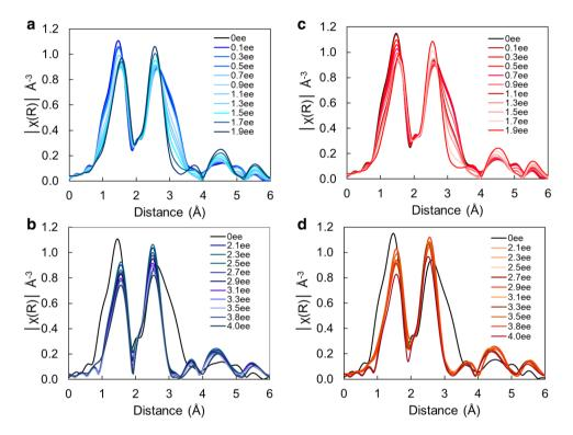
Figure 9: EXAFS spectra of Li/Fe<sub>3</sub>O<sub>4</sub> operando cell with (a), (b) EC and (c), (d) FEC electrolyte from (a), (c) 0 to 1.9 ee and (b), (d) 2.1 to 4.0 ee EXAFS plots are not corrected for phase shifts. Interatomic distances shown are ~ 0.4 Å less than true interatomic distances determined by EXAFS fitting.
