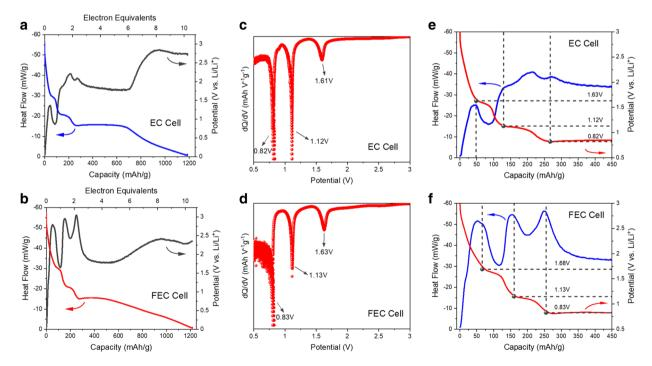
**Figure 4:** First lithiation voltage and heat flow profiles for Li/Fe<sub>3</sub>O<sub>4</sub> cells containing (a) 1 M LiPF6 EC/DMC (3/7 v/v) and (b) 1 M LiPF6 FEC/DMC (3/7 v/v) electrolyte. \*Negative heat flow represents an exothermic process. First lithiation (c) and (d) differential capacity and (e) and (f) heat flow profiles of EC and FEC-containing cells, respectively.
